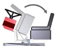
The driving station is supported on silent blocks, it can be easily rotated for inversion of the driving direction. The driving station is provided with adjustable suspensioned seat and duplicated number of pedals for both driving directions.
